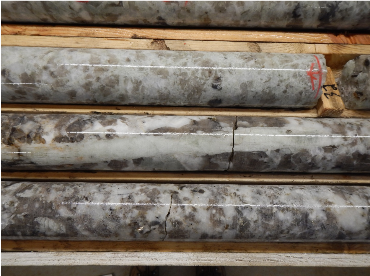
Figure 6 PWM-17-09 Main Dyke 42 cm long spodumene blade near 32 m.
