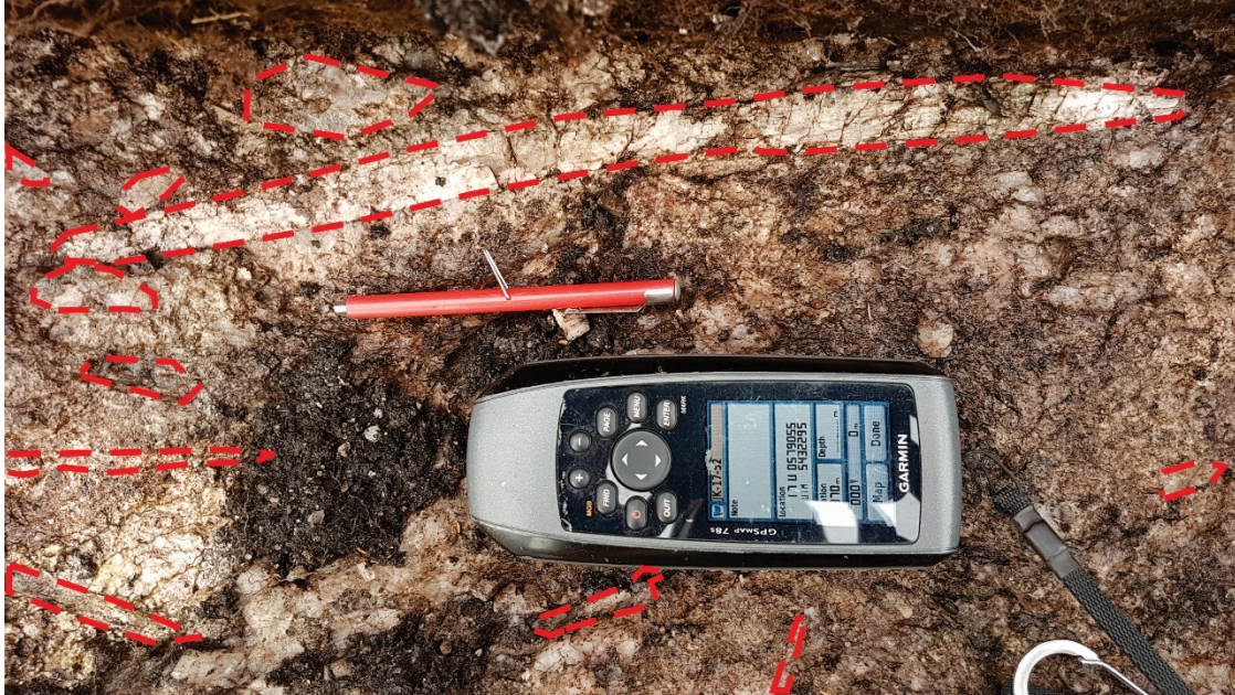
Figure 1 32 cm by 2 cm spodumene crystal in Northeast Dyke – south outcrop (sample 529463)
