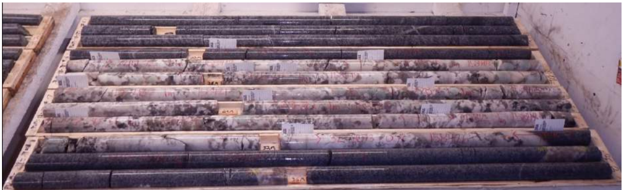
Figure 1 PWM-18-71, Boxes 5-8, 18.2-35.8 m. Note coarse-grained pale green spodumene inner intermediate zone in boxes 6 and 7.
