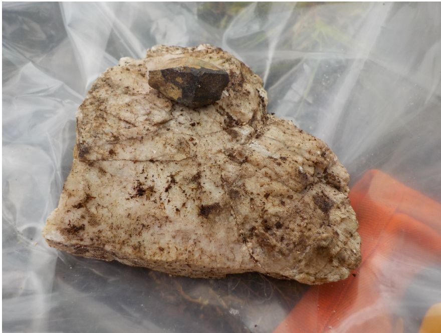
Figure 4 large Ta-oxide crystal on albite, sample 159254, Gullwing North outcrop
