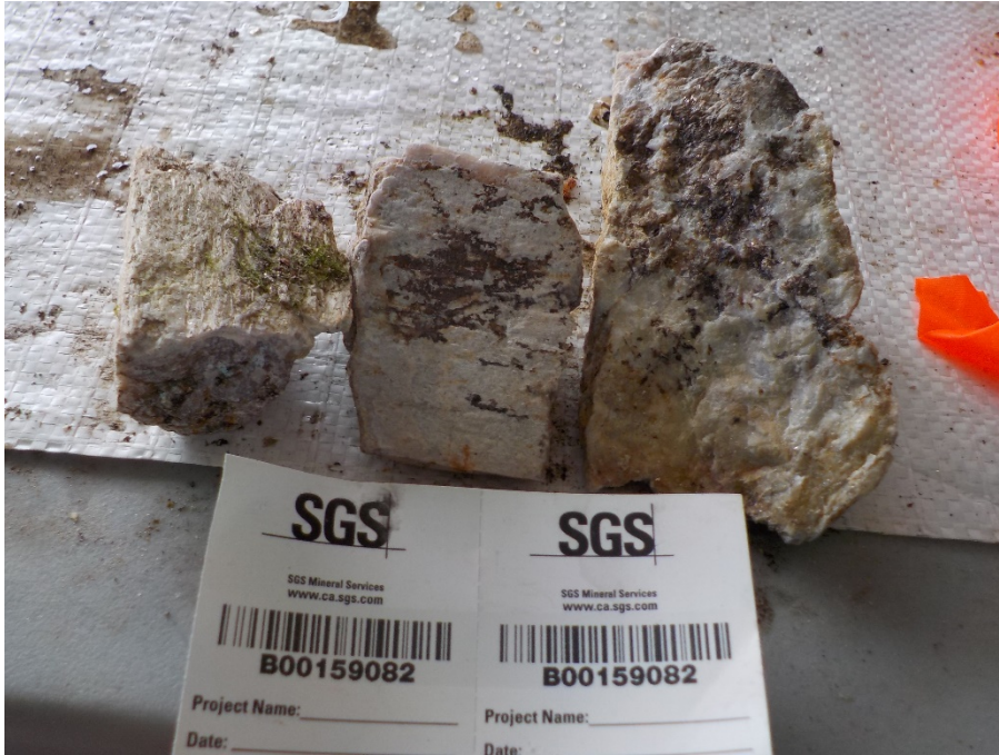
Figure 3 pure spodumene sample with trace lepidolite, sample 159082, Gullwing North outcrop
