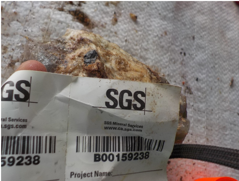
Figure 2 coarse-grained Ta-oxide in albitized K-feldspar zone, sample 159238, Tot Lake
