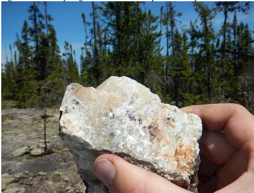
Figure 3: Photo of purple lepidolite (Li-mica) from 10 m wide dyke near the spodumene dyke on Dome 9, Case Lake.
