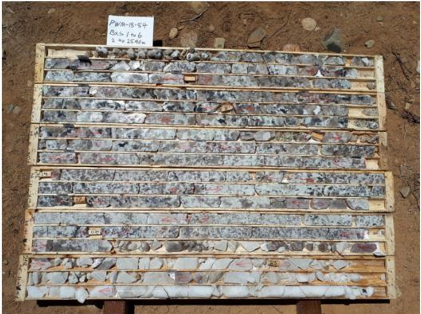
Figure 1 PWM-18-84, boxes 1 to 6, spodumene pegmatite with up to 10% spodumene (boxes 1 to 5) and quartz core (box 6), Main Dyke, Case Lake.
