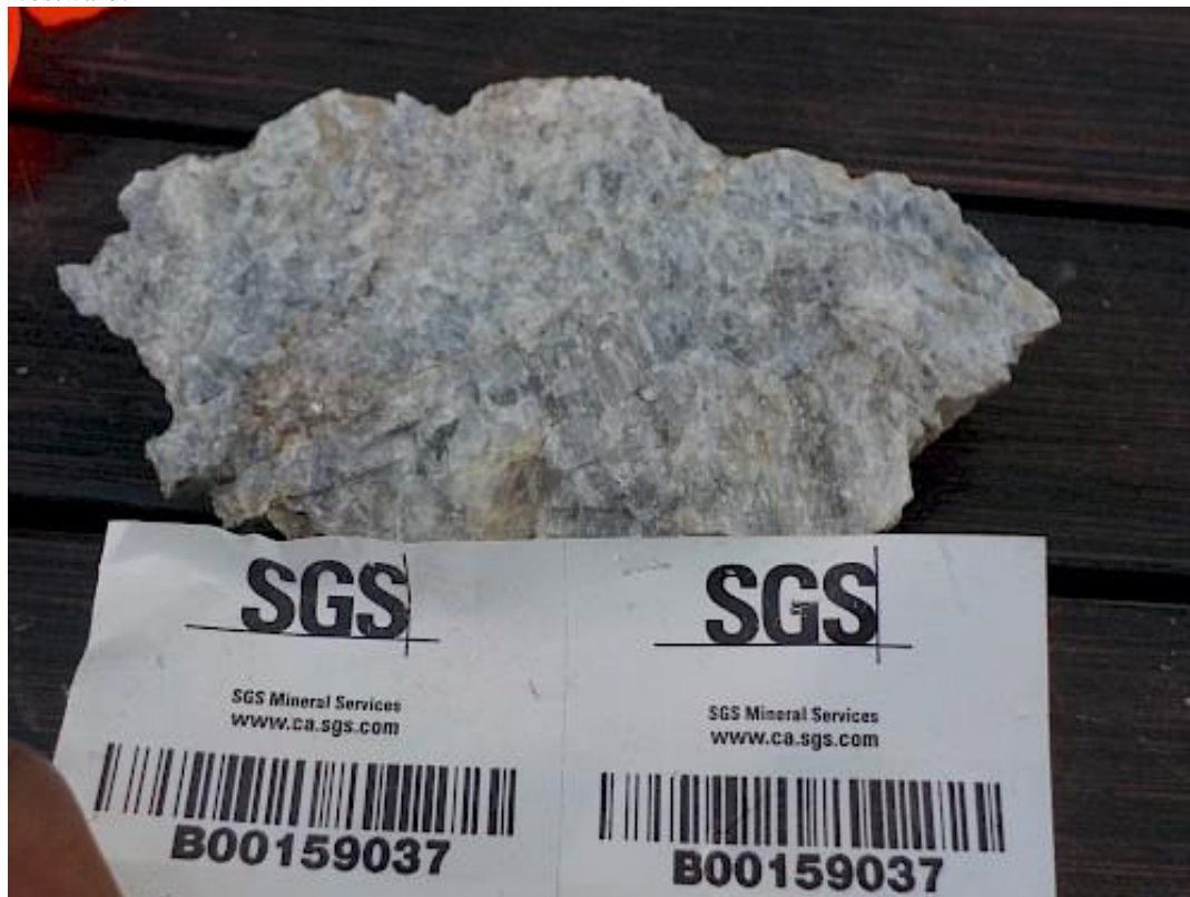
Figure 1 Grab sample 159037 of pure petalite from the western extension of Marko’s pegmatite, Paterson Lake Property, Ontario.
