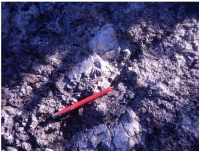
Figure 2 Pale green spodumene crystals next to white K-feldspar in the East Dyke.
